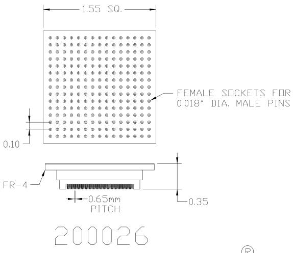
144 PIN, .65mm, TQFP DELTA Probe DIMENSIONS ARE IN INCHES
